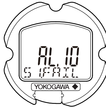
Figure 6.1 Integral Indicator with Error Code
