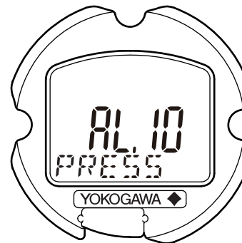
Self-diagnostic error on integral indicator (Faulty transmitter)
